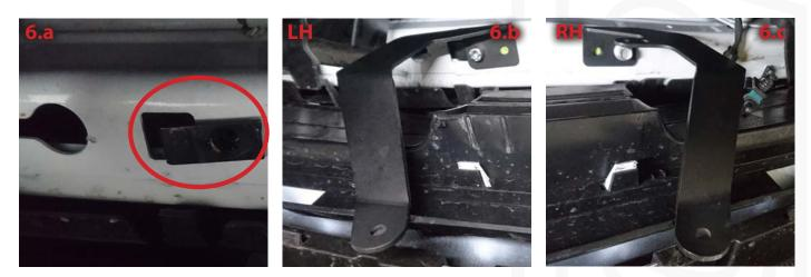
Note - MY18 cars and onwards mount the LH bracket on top of the radar mount.
