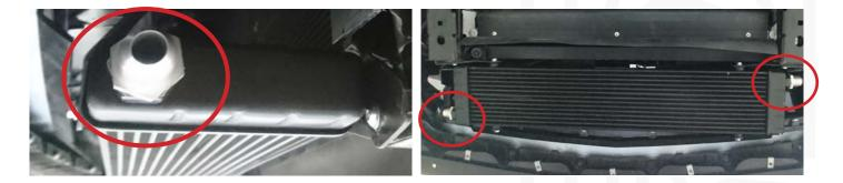
12. Route and connect the hoses onto the just installed fittings as per image below, ensure that the hex fitting on the oil cooler is supported with a correct sized spanner to prevent it from twisting on the tank. Note - RH side air seal may need some trimming.
