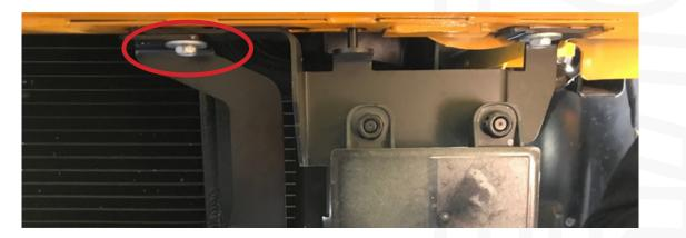
7. Insert the 2 U nuts into the lower front rails as per images 7.a and 7.b below. Mount the rear oil cooler mounting brackets as per image below but leave them lose. Note 'S' bend is to point forward - see image 8.a.
